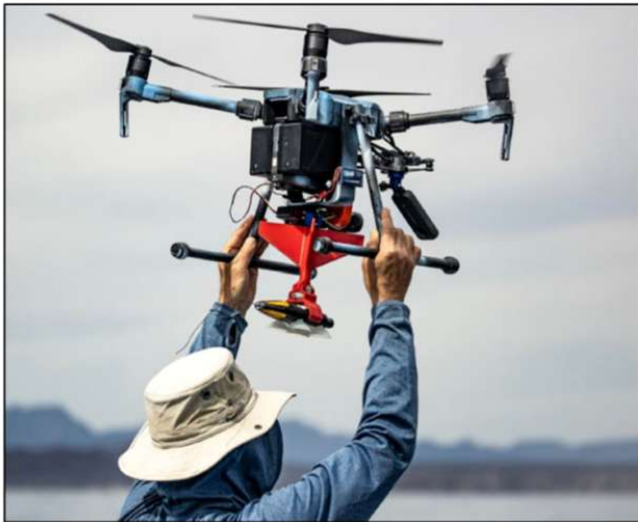
Figure 2. (a) Hand launching assembled M210 V2 with the DTAG deployment package. (b) DTAG drop system components.
