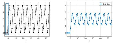
Filter processes samples to enhance signals, e.g., freq.-selective filter removes unwanted frequencies, leaving desired signal alone
