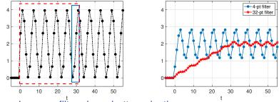
Longer lowpass filters have better rejection ... but they take longer to respond to changes in input Filter processes samples to enhance signals, e.g., freq.-selective filter removes unwanted frequencies, leaving desired signal alone
